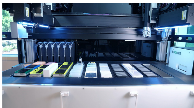
Figure 3: The Stuntman deck staged with reaction, quench, and analysis plates during a closed-loop run.
