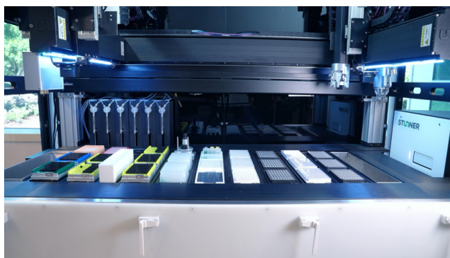
Figure 5: The Stuntman deck staged with reaction, quench, and analysis plates during the closed-loop run.
