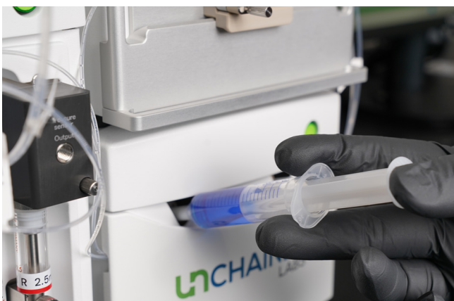
Figure 3: Loading the sample loops with reagent ahead of running an automated set of experiments.
