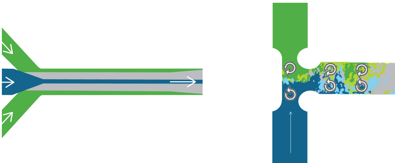
Figure 4: Comparison of stable laminar flow mixing (left) and chaotic mixing (right).
