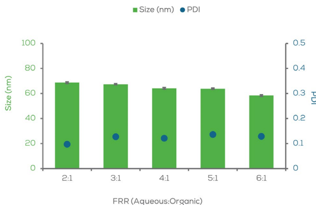
Figure 4: mRNA-LNPs produced by various FRR (aqueous to organic phase) at a fixed TFR of 5 mL/min with no dilution. LNPs ranged from 58 nm to 68 nm post-dialysis, with an average PDI of 0.12. Particle size distribution and polydispersity index (PDI) were determined by dynamic light scattering (DLS). The error bars represent standard deviation of the mean n=3.
