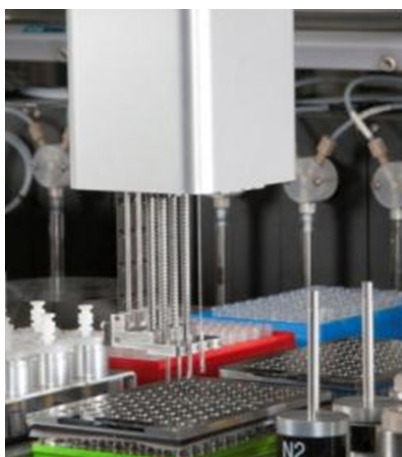
Heated 4-tip liquid dispenser – fixed pitch – extended tip
