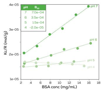
Figure 10: Scattering intensity as a function of BSA concentration over pH 4–7, and the calculated  ${\sf B}_{22}$  values for each condition.
