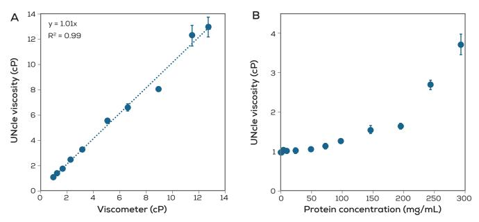
Figure 12: Correlation of glycerol standards measured on Uncle and a viscometer (A), and the viscosity of a protein at increasing concentration as measured by Uncle (B).
