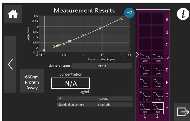
Figure 4: Illustration of the Results screen on the Little Lunatic. Reference samples (shown as yellow crosses) are used to create a standard curve and concomitant equation to calculate the concentration of protein samples (gray squares, red if selected).
