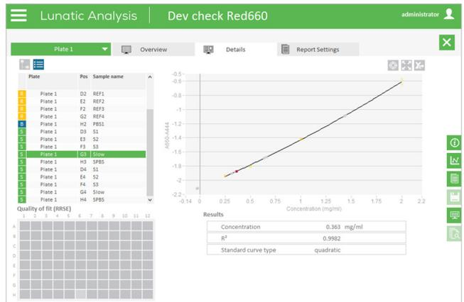
Figure 3: Illustration of the Results screen on the Lunatic. Reference samples (shown as yellow crosses) are used to create a standard curve and concomitant equation to calculate the concentration of protein samples (gray squares, red if selected).
