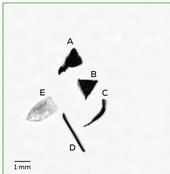
Figure 2: Mosaic image captured by automatically scanning an adhesive round at 10x. The five particles analyzed can clearly be seen. A: Syringe needle fragment. B: Crimp cap particle. C: Bottle cap fragment. D: Piece of copper wire. E: Glass shard. LIBS spectra were acquired for each particle and compared to the Hound built-in reference database.
