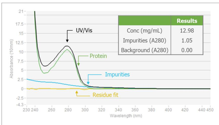
Figure 4: Deconvoluted absorbance spectrum of BSA using the Total Protein application on Big Lunatic. The table (inset) lists the results reported from the Unmix algorithm, including the protein concentration, impurities and background absorbance at 280 nm.
