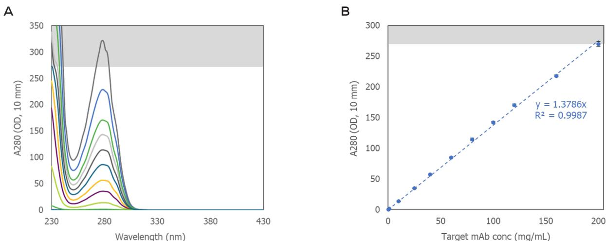
**Figure 3:** Spectral results for a monoclonal antibody from 0.1 to 200 mg/mL measured on Big Lunatic. **A:** The full spectrum of each mAb concentration, overlaid. **B:** The average OD values of the extrapolated IgG spectrum is plotted as a function of the target protein concentration. The grey area indicates the upper limit of the linear range of Lunatic. Error bars denote the standard deviation of four replicate measurements.
