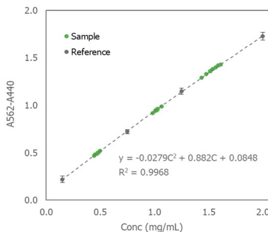
Figure 5: Samples overlaid on a standard curve generated using the BCA application on Big Lunatic. Measured sample concentrations are consistent with the serial dilution preparations. Error bars denote the standard deviation of octuplicate measurements.
