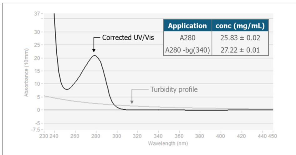
Figure 2: Absorbance spectrum of BSA using the A280 Protein application on Big Lunatic. The table (inset) compares the concentrations calculated using turbidity subtraction and conventional single-wavelength subtraction methods.
