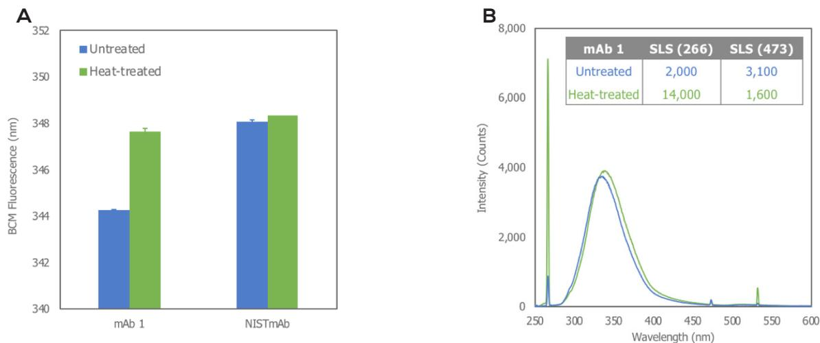
Figure 2: **A**: Intrinsic fluorescence of mAb1 and NISTmAb, with or without a heat treatment. **B**: Fluorescence emission spectrum of mAb1. The SLS intensity counts at 266 and 473 nm are shown in the inset table.
