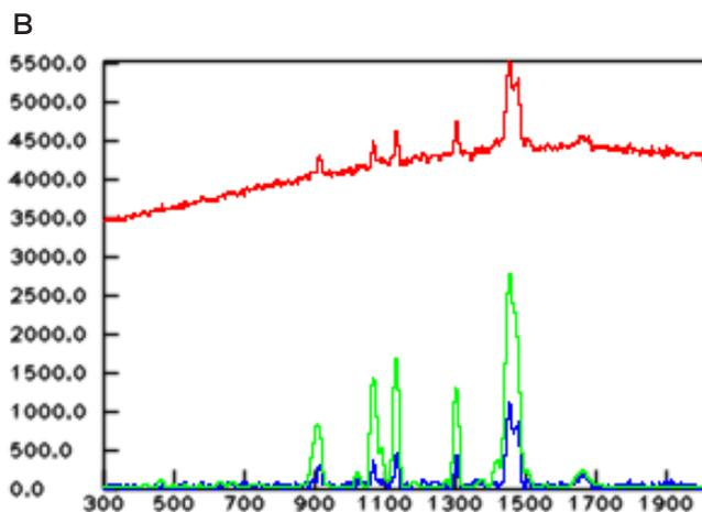
Figure 4: (A) 50x microscopic image of a 100 μm lauric acid particle. (B) Raman (532 nm), 10s spectrum of the 100 μm lauric acid particle (red original, blue optimized, green database match).
