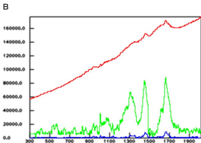
Figure 3: (A) 50x microscopic image of a 60 μm protein aggregate. (B) Raman (532 nm), 30s spectrum of the protein aggregate (red original, blue optimized, green database match).
