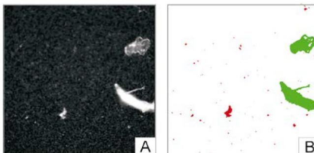
Figure 3: (A) Dark field image of one 500  $\mu\text{m}$  x 500  $\mu\text{m}$  field. (B) Image analysis highlighting measured particles (green) and all other particles (red).
