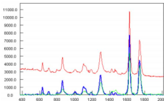
Figure 3: Chemical identities are confirmed by processing a raw Raman spectrum (red) to create a processed spectrum (blue) to match to an expandable reference library (green).
