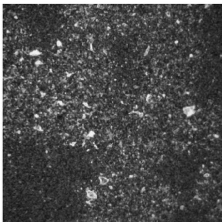
Figure 2: Dark field image of DPI particulates collected on the filter round.
