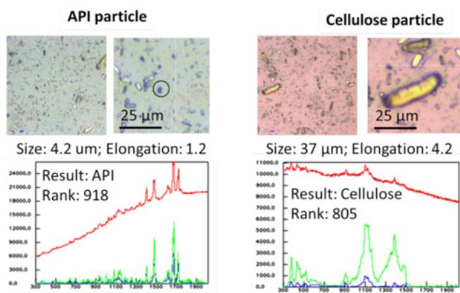
Figure 2: **Left:** Images of API particles and Raman spectra for a particle showing the matched reference spectra for the API. **Right:** Images of cellulose particles and Raman spectra for a particle showing the matched reference spectra for cellulose. Overall, API particles are much darker and rounder than cellulose particles.
