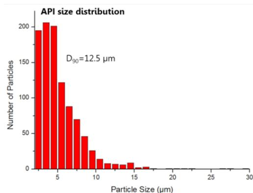
Figure 4: Size distribution of 1,011 API particles analyzed by Hound in 4 hours. Average particle size is 5.2  $\mu\text{m}$  and D90 is 12.5  $\mu\text{m}$ .
