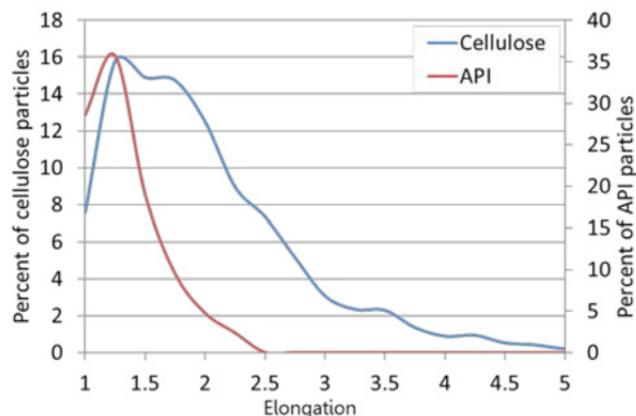
Figure 3: Elongation distribution of API and cellulose particles. Elongation values for API particles are lower than those for cellulose particles, which is useful for selective analysis.
