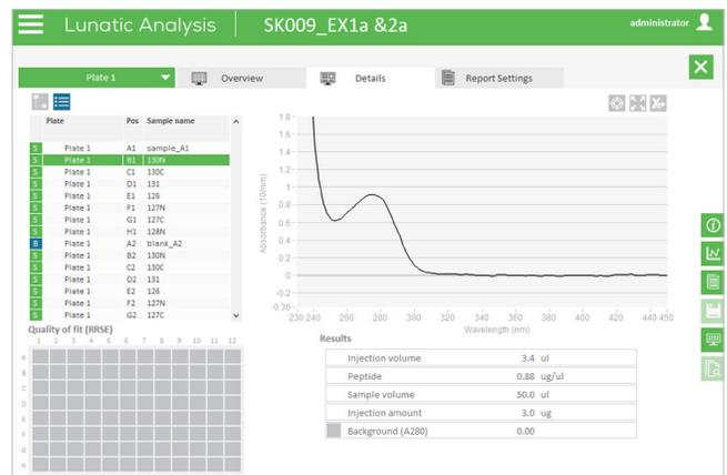
Figure 3: Illustration of the Results screen on the Big Lunatic. In addition to the injection volume, the peptide concentration is also displayed.
