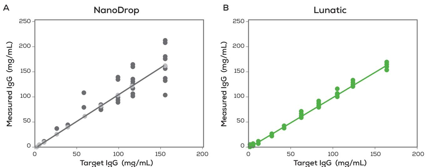
Figure 3: Results for a gravimetrical IgG dilution series on four NanoDrop (A) and four Lunatic (B) instruments.
