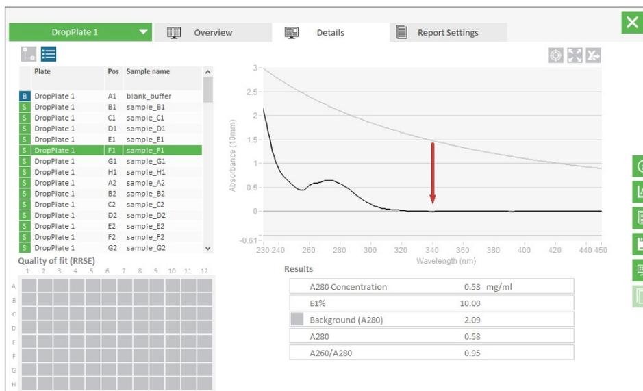
Figure 2: Turbidity correction. The Lunatic platform performs a turbidity correction that takes into account wavelength-dependent scatter profiles (gray line on the graph) rather than choosing the absorbance at one specific wavelength (e.g., 340 nm) to correct the entire UV/Vis spectrum.
