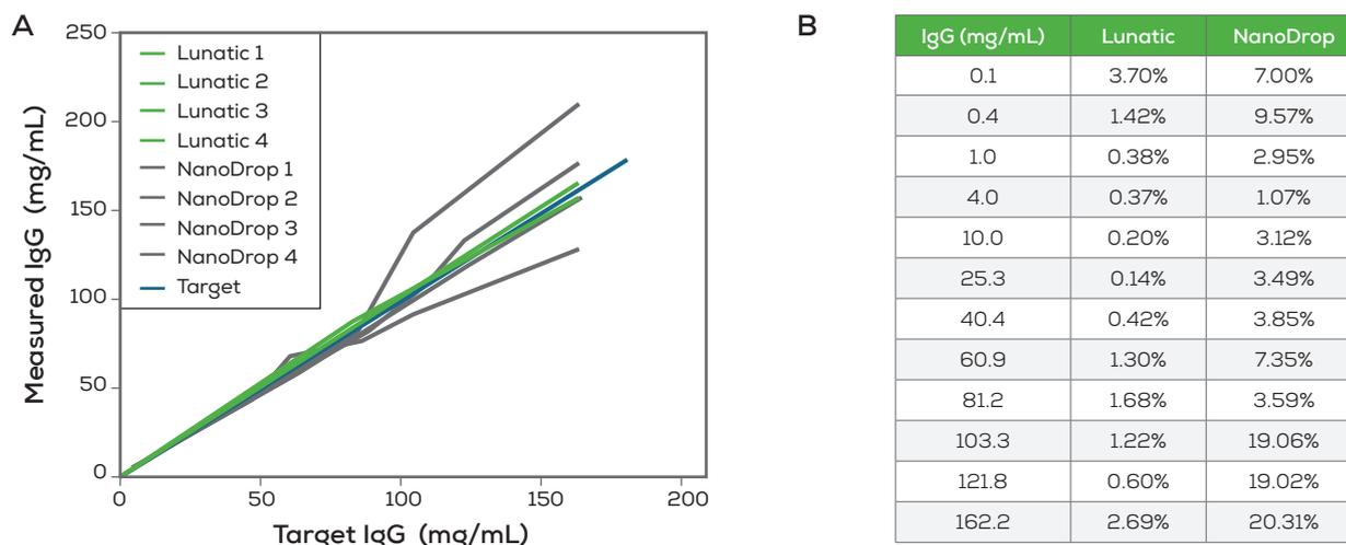
Figure 4: (A) Comparison of the average concentrations per instrument. NanoDrop and Lunatic instruments are represented by gray and green lines respectively, target concentration is annotated by a blue curve. (B) The percentage of variation among instruments.
