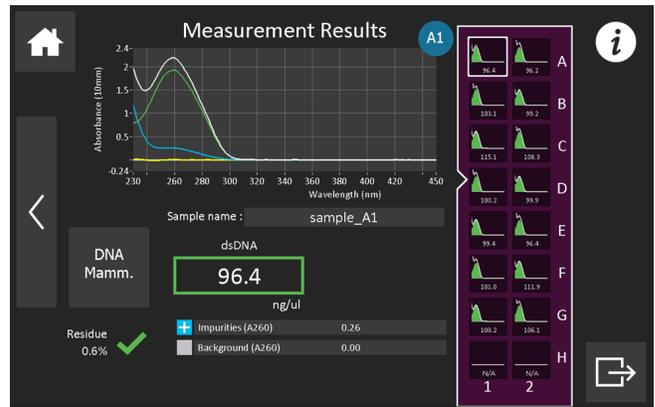
Figure 4: Illustration of the Results screen on the Little Lunatic. Unmix app results of the selected sample are shown as spectral shape as well as in calculated values. Additional impurity and/or background detailing will be reported if possible.
