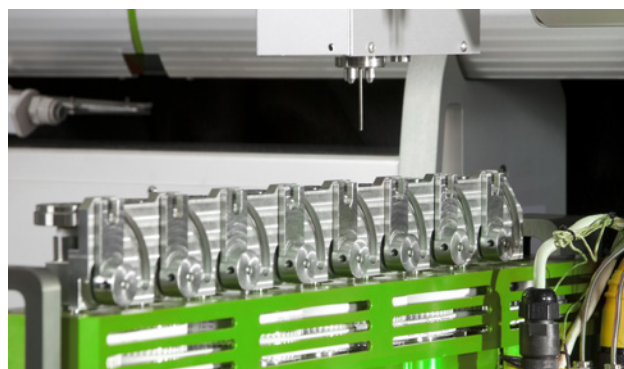
Optimization sampling reactor (OSR)
