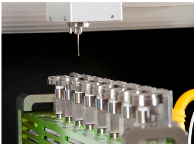
Figure 2: The OSR with controlled atmosphere sampling port technology.
