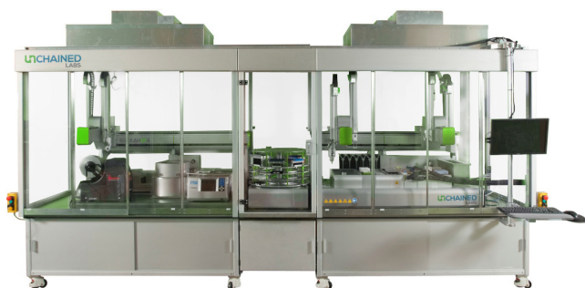
Figure 1: The Big Kahuna system configured for biologics formulation.
