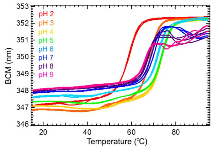
Figure 3: BCM versus temperature plots for HEWL in pH 2 - 9 buffers.
