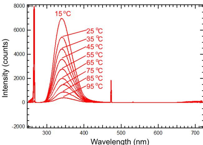
Figure 2: Intrinsic fluorescence emission spectra for HEWL in pH 6 buffer between 15 and 95 °C.
