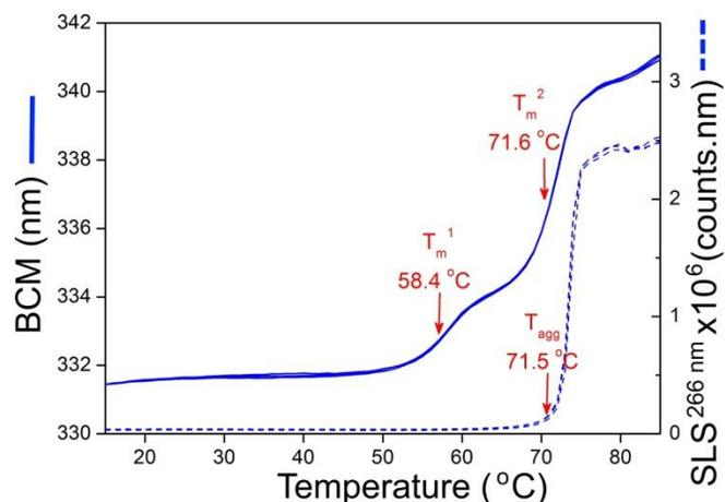
Figure 7: Overlay of intrinsic fluorescence and SLS data obtained during a thermal ramp of MAb1 at pH 4.6. The  $T_m$  and  $T_{agg}$  values extracted from this data are displayed in red.
