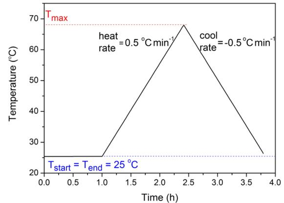
Figure 1. Sawtooth temperature cycle profile.
