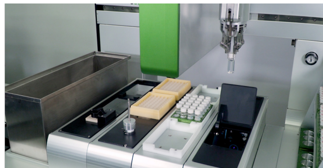
Figure 1: Big Kahuna or Junior (pictured) with VIS automates sample analysis, and quantifies color, visible particle count, and turbidity of biologics non-destructively.
